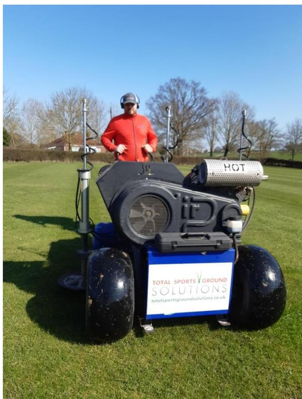
This clever piece of machinery injects air under pressure laterally into the ground at a depth of 6 and 12 inches, reducing compaction, encouraging drainage and promoting root growth.
